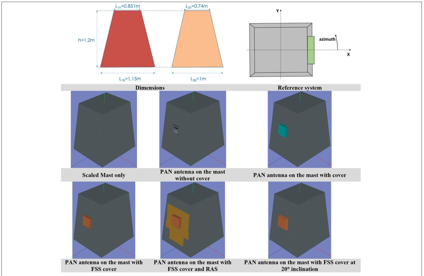
(c) - Geometry of the simulated configurations: the metal is shown in gray, the dielectric with  $\epsilon_r$  of 3.5 is in light blue, the FSS film in orange and the RAM structure in mustard
