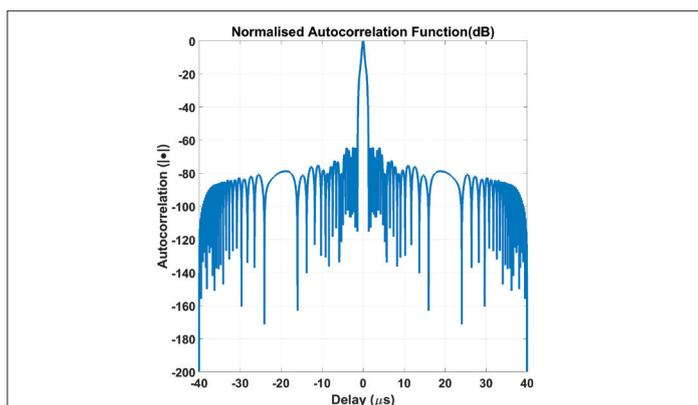
(c) - Normalized ACF for  $T=40ms$ ,  $B=5MHz$
