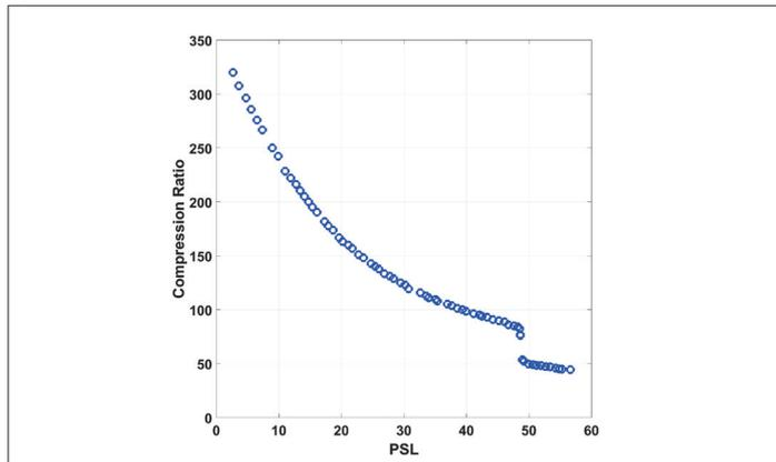
(a) - Pareto fronts of the compression ratio of the compressed waveform versus PSL (Peak to Sidelobe Level) for a Bandwidth-Duration product  $BT=200$ . Raised cosine weight at the receiver with roll-off factor 0.1 and a number of sinusoidal components of the ACF spectrum  $N=5$ ;
