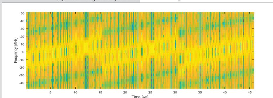
(b) PRBS (pseudorandom binary sequences) modulated FMCW waveform, 30MHz noise bandwidth. The typical "ramp" of FMCW signal is completely masked by the noise, leading to pseudo random noise like waveforms and, hence, LPI operations
