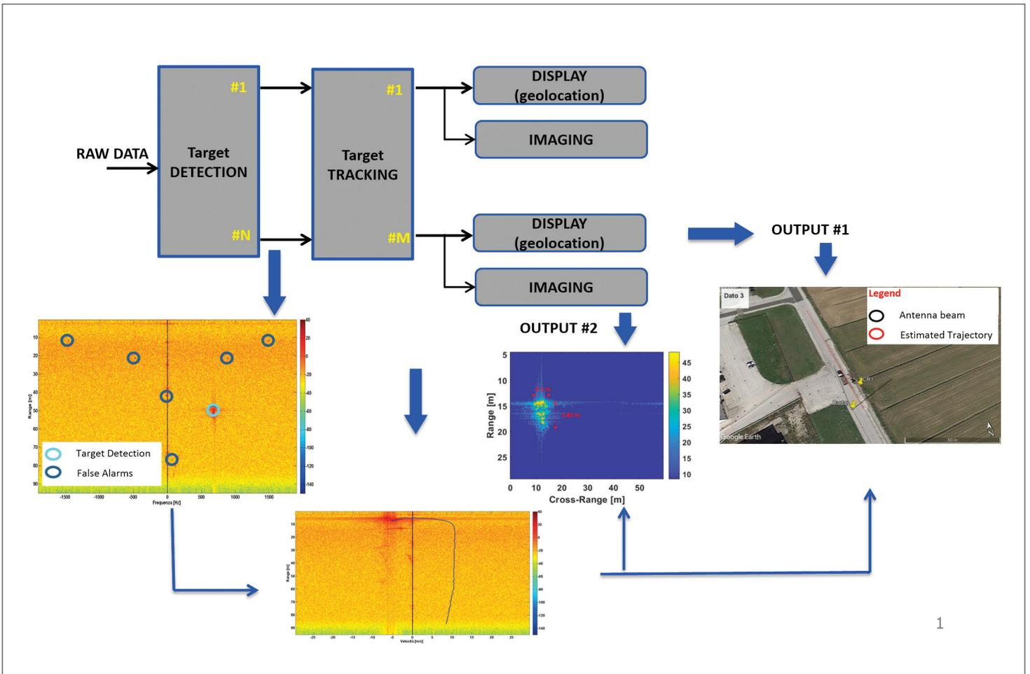
(c) - Processing Block Diagram and relative output
