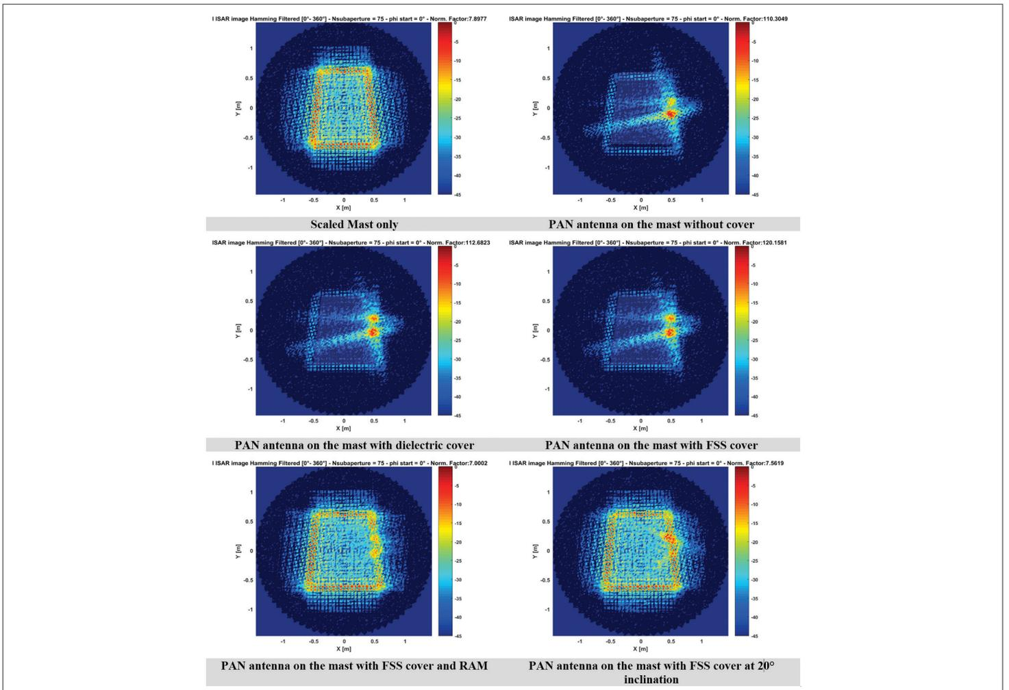
(d) - Final ISAR images of all configurations on the plane  $\varphi = 0^\circ$  in polarization V. The images have the same dynamic range but are normalized to a different maximum value identified as NF (Normalization Factor)
