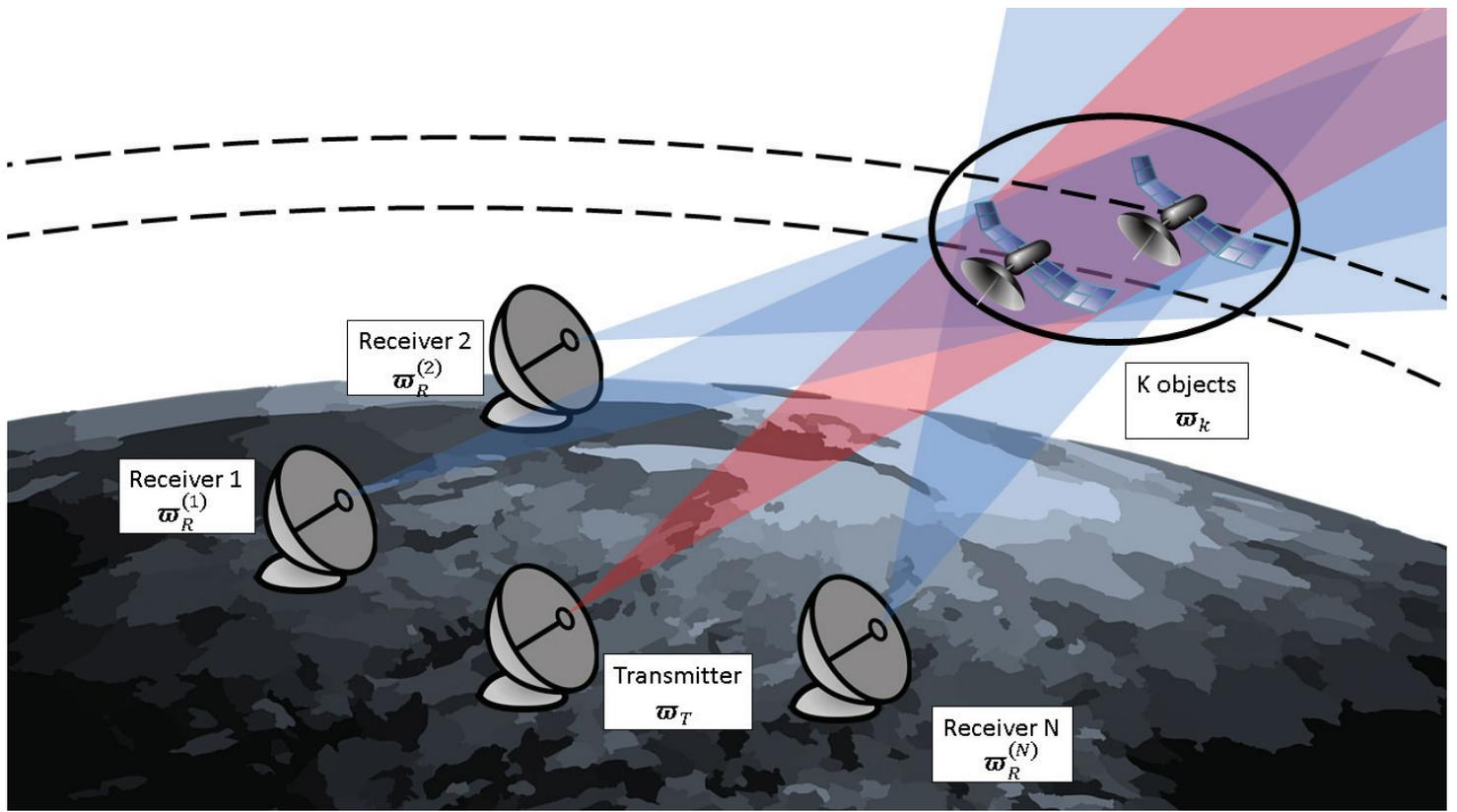
(b) - Multi-bistatic radar configuration for RSO orbit determination
