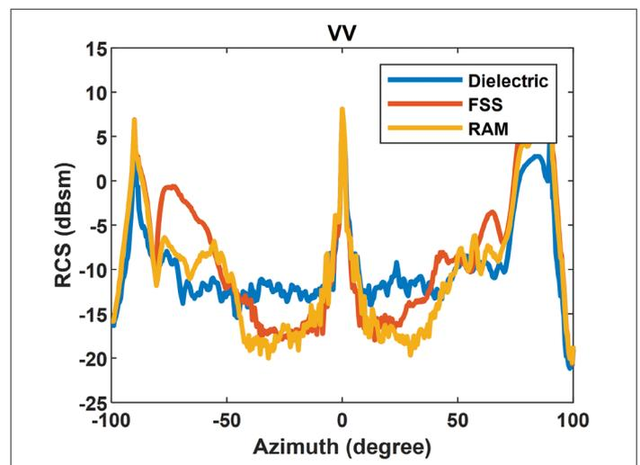
(b) - Comparison of simulated measurements of the measured RCS averaged on the 18-26 GHz band. Measured RCS averaged on the 18-26 GHz band: comparison of the countermeasures using FSS and RAM compared to the dielectric cover only
