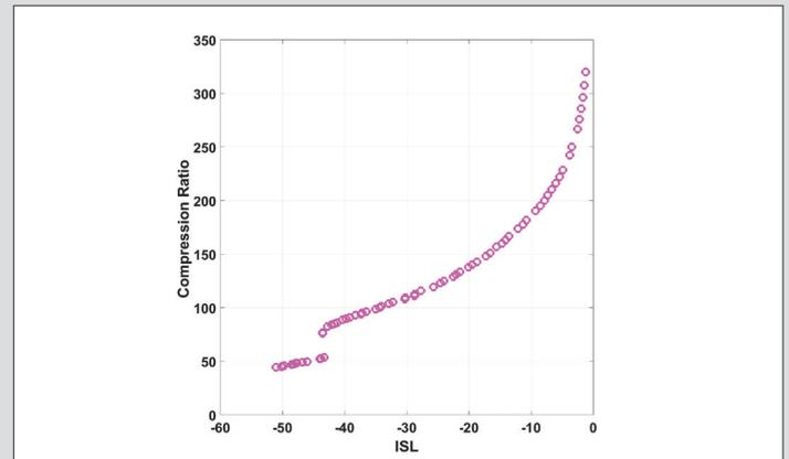
(b) - Pareto fronts of the compression ratio of the compressed waveform versus ISL (Integrated Sidelobe Level) for a Bandwidth-Duration product  $BT=200$ . Raised cosine weight at the receiver with roll-off factor 0.1 and  $N=5$
