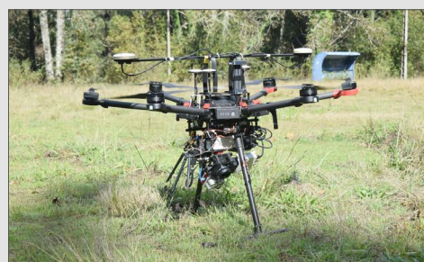
(b) POSEIDON system. The drone payload (EO/IR camera, radar sensors IMU system and GPS antenna) has been integrated successfully in the DJI matrice 600 pro
