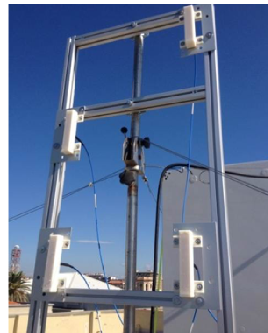
(a) The first ground based interferometric radar system developed at the RaSS laboratory in 2016 - PIRAD demonstrator
