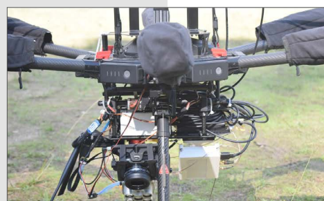
(c) A detail of the integration showing the radar antenna and EO/IR camera pointing toward the same direction
