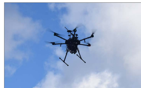
(d) First flight of the POSEIDON system to test the system integration and endurance before measurements
