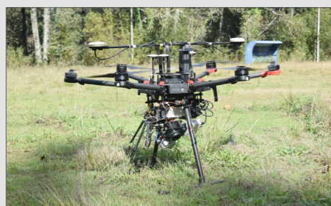
(b) POSEIDON system. The drone payload (EO/IR camera, radar sensors IMU system and GPS antenna) has been integrated successfully in the DJI matrixe 600 pro
