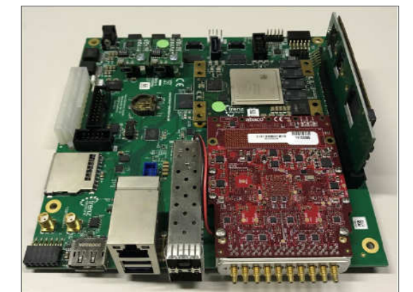
(g) Radar digital component. It generates the waveform, acquires the receiving signals and communicates with the 4G router;
