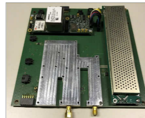
(h) Front-end module. It allows transmission of a LFM CW signal with a bandwidth of 600 MHz around 9.6 GHz;
