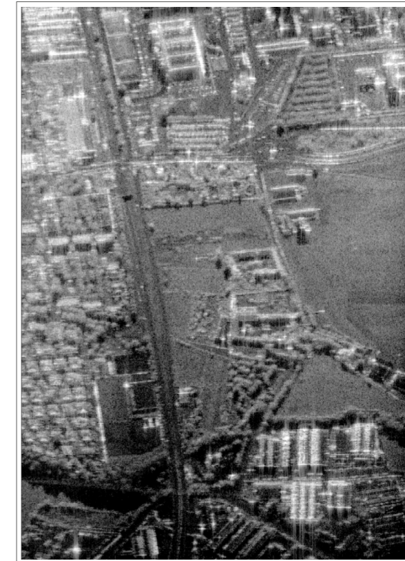
(e) SAR image of the illuminated area formed with BackProjection algorithm
