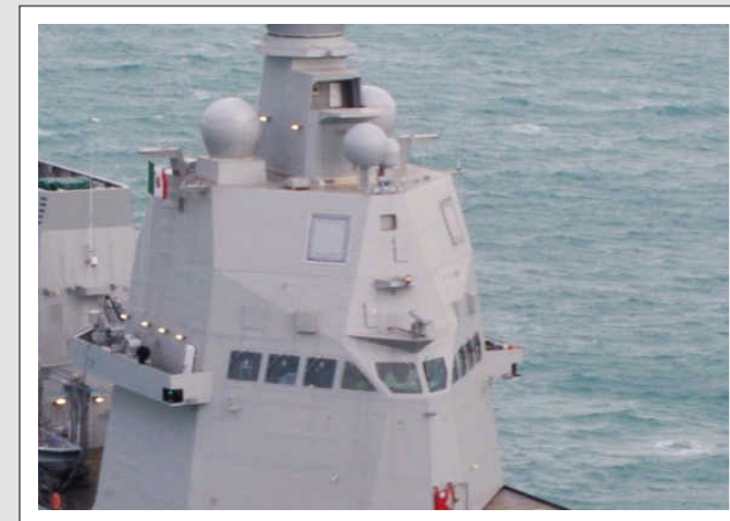
(c) View of the Paolo Thaon Revel (P430) vessel with CNIT installed antennas during test;
