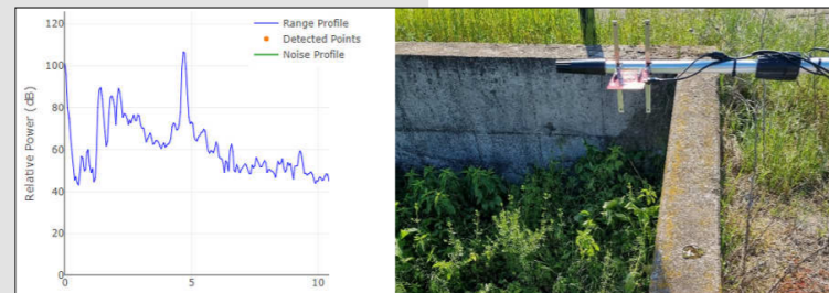
(b) Signal received. The central peak corresponds to the power received from the water surface, the main peaks on the left correspond to the power received from the concrete abutment of the bridge
