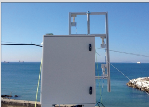
(a) The first ground based interferometric radar system developed at the RaSS laboratory in 2016 - PIRAD demonstrator
