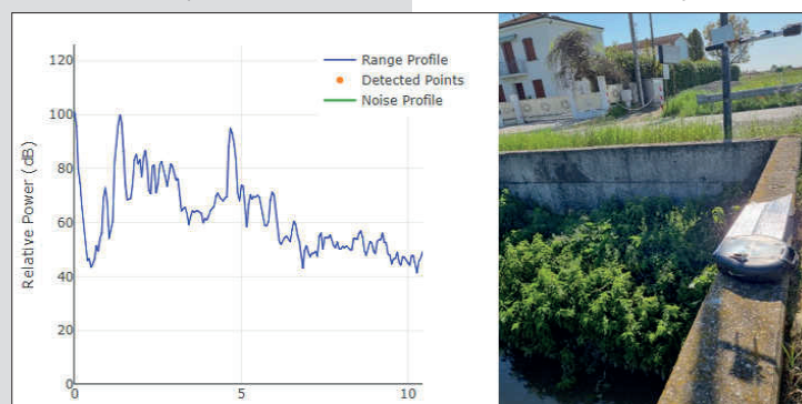
(c) Signal received. The central peak corresponds to the power received from the water surface, the main peak on the left correspond to the power received from the reflecting panel placed on the concrete abutment of the bridge.
